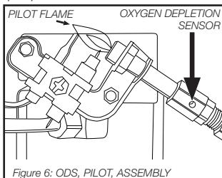
8. Inspect and clean pilot (mounted to bracket) by using a vacuum or apply air pressure through the holes in the pilot indicated by the arrows in Figure 6. **WARNING:** Never use needles, wires, or similar cylindrical objects to clean the pilot to avoid damaging the calibrated orifice that controls the gas flow.
